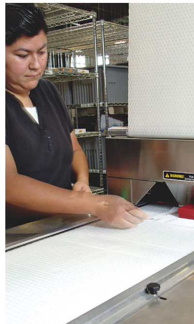
An operator checks an item moving through the packing machine on the bottom web of cushioning/shipping material from a roll.
